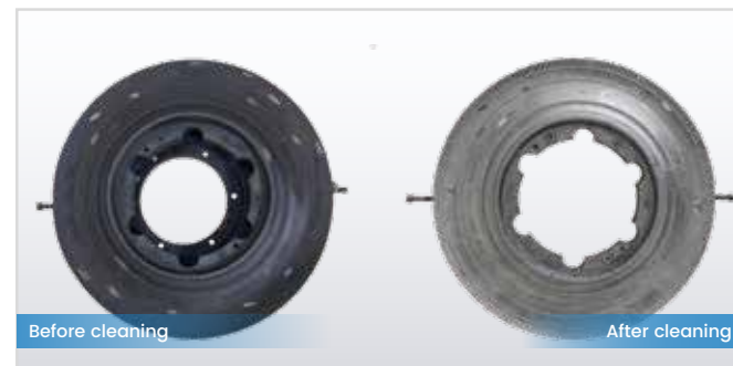
Clean tyre mold
